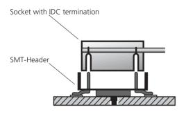
2.) Transition connector soldered directly to the circuit board
