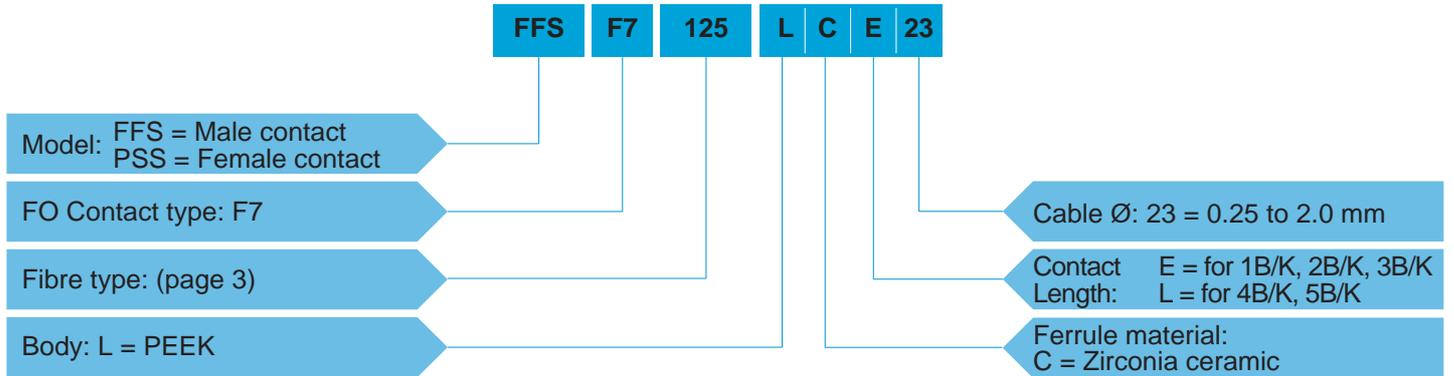
**FFS.F7.125.LCE23** = Male F7 type fibre optic contact, ferrule bore diameter of 125 µm, PEEK body, Zirconia ceramic ferrule, contact length for 1B/K, 2B/K or 3B/K series, for cable with diameter max = 2.0 mm.
