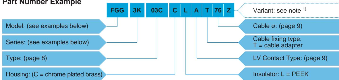
**FGG.3K.03C.CLAT76Z** = Straight plug with key (G), 3K series, multi-fibre type to accept 4 F7 type fibre optic contacts, chrome-plated brass housing, PEEK insulator, cable fixing type T for 7.5 mm diameter cable, and nut for fitting a bend relief.
