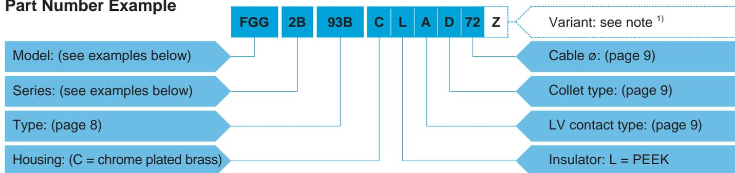
**FGG.2B.93B.CLAD72Z** = Straight plug with key (G), 2B series, mixed type to accept 2 F7 fibre optic contact and 4 low voltage electrical contacts, chrome-plated brass housing, PEEK insulator, 4 male solder electrical contacts, type D collet to suit a 7.0 to 6.1 mm diameter cable, and a nut for fitting a bend relief.
